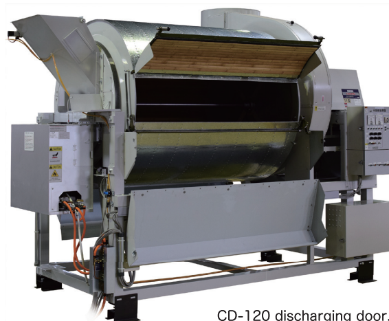
CD-120 discharging door, front cover opened
